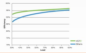
Improved efficiency of the NO-BREAK KS\*7 **2** with variable cooling vs. other Diesel Rotary UPS systems.
